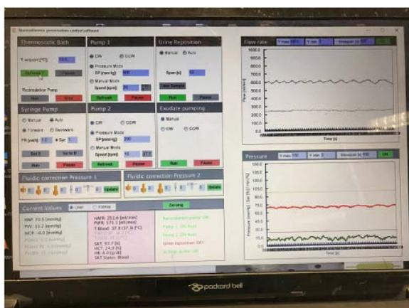
Figure 3. Software interface developed for system configuration and control while monitoring the adjustable and non-adjustable key variables for the normothermic perfusion process.
